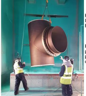
Resicoat R4 is a WRAS approved product and is a one-part, heat curable, thermosetting powdered epoxy coating that provides maximum corrosion protection of line pipe and fittings.
