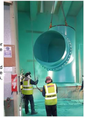
The epoxy coating is unaffected by soil forces and is highly resistant to moisture penetration, bacteria and fungus attack, soil acids, alkalies and salts and other chemicals associated with underground and underwater use.
