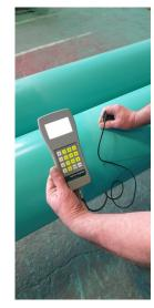
Thickness check, Resicoat R4 applied to 300 microns Minimum standard coating thickness, or to a requested minimum to align with customer requirements or specification.
