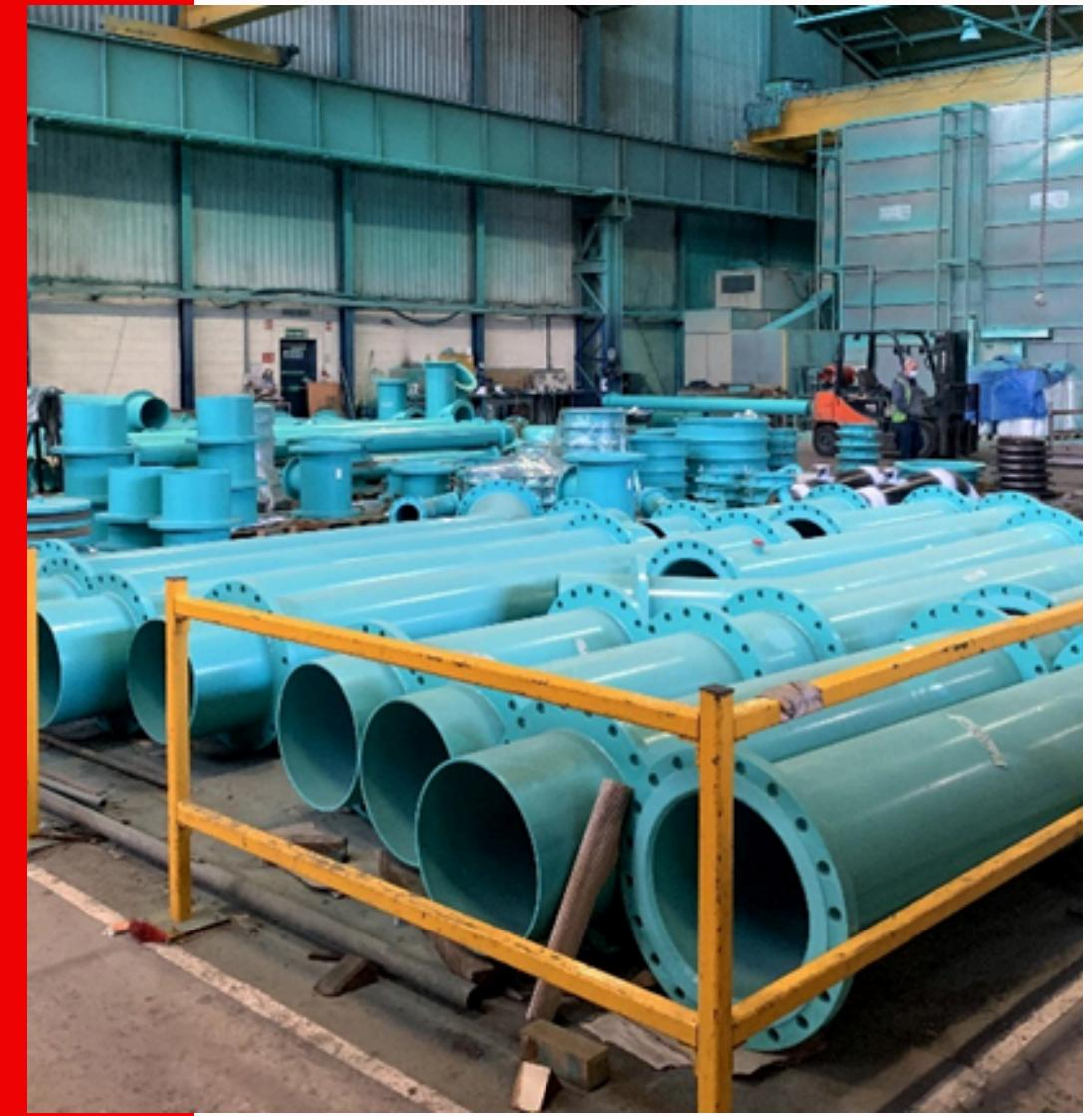
The epoxy coating is unaffected by soil forces and highly resistant to moisture penetration, bacteria and fungus attack, soil acids, alkalies and salts and other chemicals associated with underground and underwater use.
